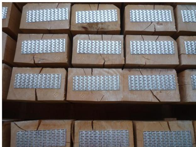
**3.1.2 Dry cracks (beech, cut single and dual stemmed, secured with sleeper crowns a. protective crack plates, here without stratification - additional protection with sleeper protection bands required!)**
