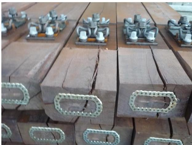
**3.1.3 Dry cracks (beech, protected with sleeper protection band)**
